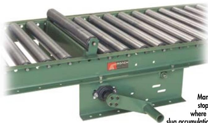
Manual operated gravity conveyor stops are hand operated and used where line control is required such as slug accumulation, indexing, workstations, etc.
